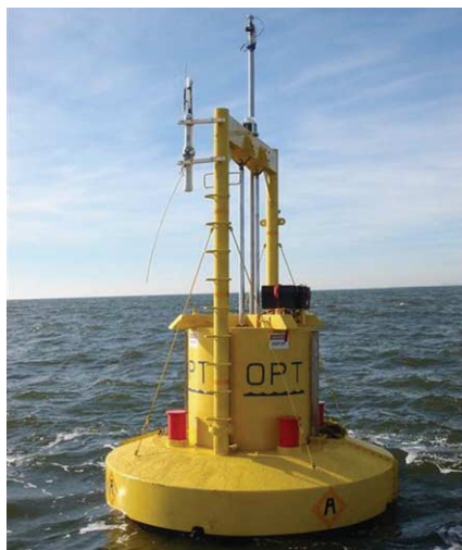
OPT's PowerBuoy (TM) which captures energy from the rising and falling of waves
